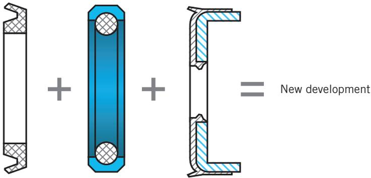
2 New development: the idea behind the transmission piston seals TCS is to combine the most favourable characteristics of each of the three individual seals in a single one
