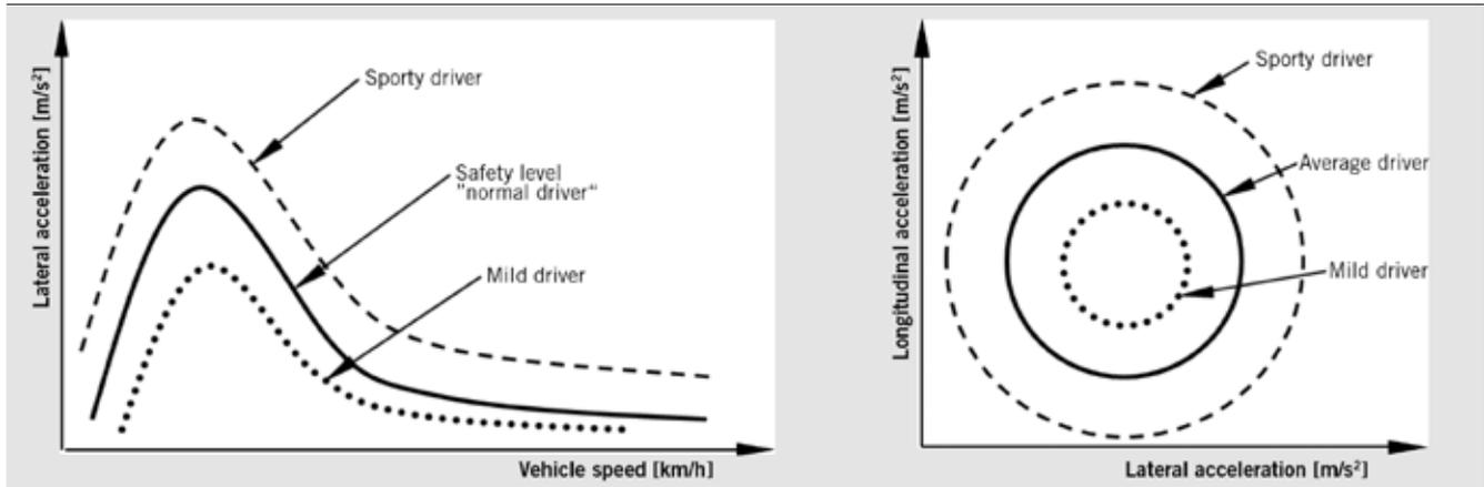
③ Reference samples regarding the correlation of vehicle speed and lateral acceleration and usage of Kamm's circle
