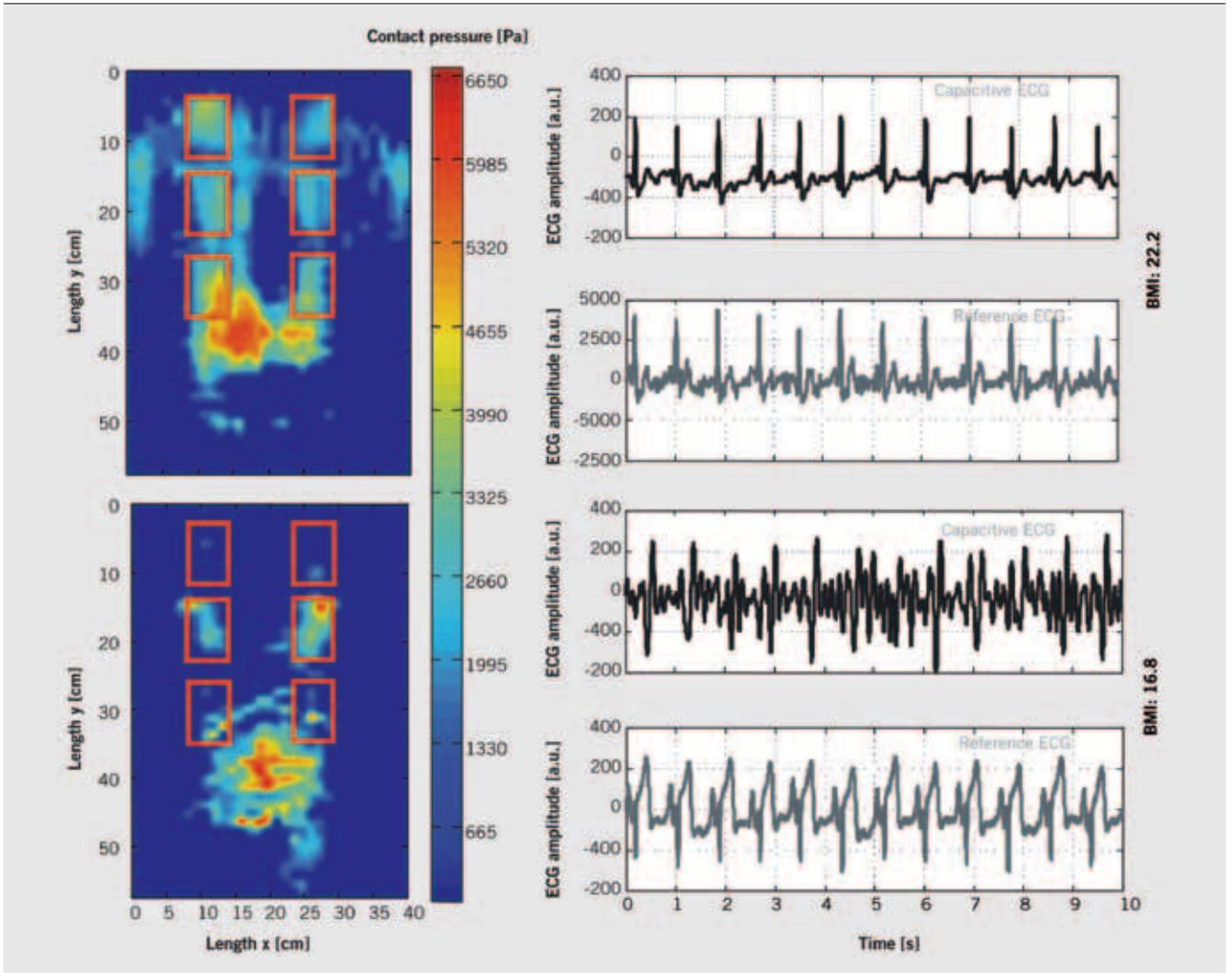
④ Contact pressures and related ECG signals for different body mass indices in artificial units [a.u.] (top: BMI in normal range, bottom: BMI below the normal range)
