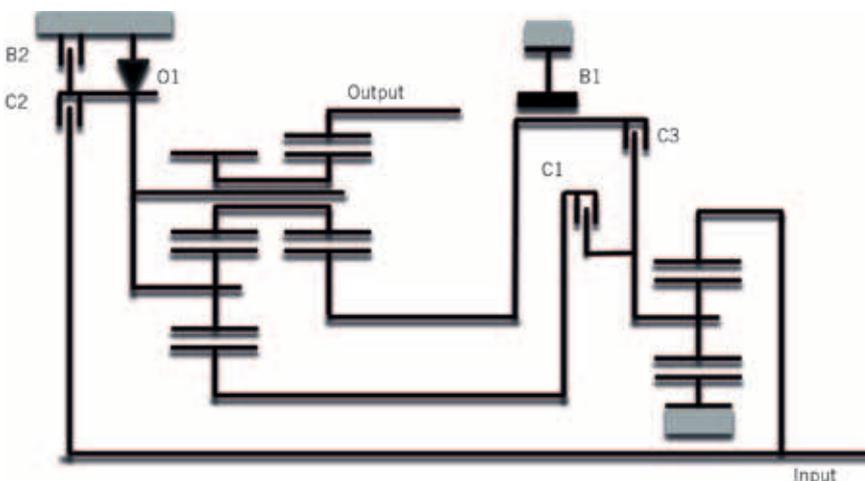
❷ Power flow of the transmission with two brakes (B) and three clutches (C) as well as one one-way clutch (O)
