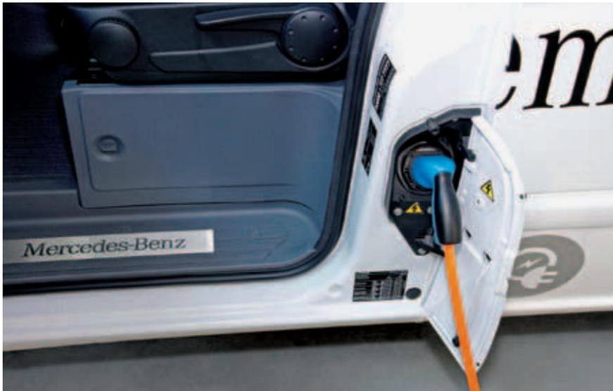
⑨ An immobilizer prevents the driver from setting the Vito E-Cell in motion during charging
