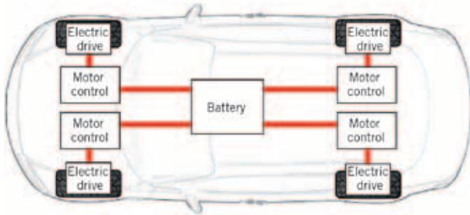
⑥ Drive-train based on four wheel-hub motors
