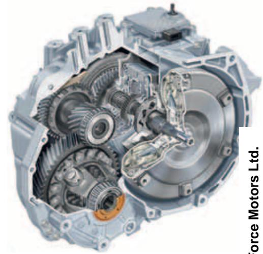
❶ Section through the new six-speed automatic transmission AF40 Gen II for 450 Nm torque
