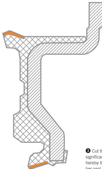
3 Cut through seal: the transmission piston seal TCS achieves significantly improved gear shift performance; key technology is hereby the combination of the PTFE layer (orange) with the rubber seal lip (checked) and the metal base element (hatched)
