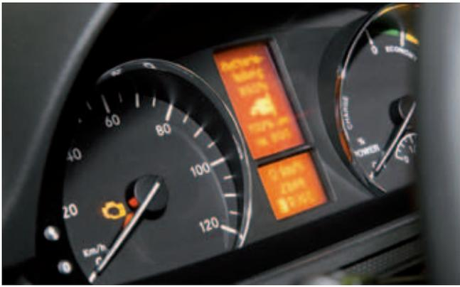
② Power output display instead of the rpm counter
