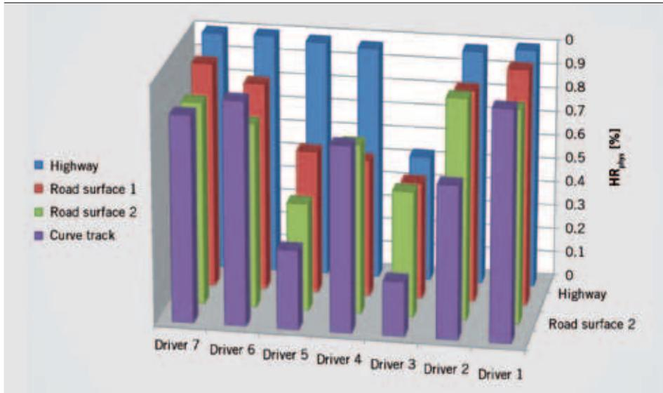
6 QRS detection rate in the physiological range for different drivers and different test tracks; extreme acceleration and curved way of driving for Driver 3
