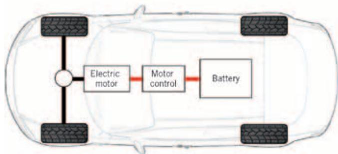
① Drive-train based on a central electric motor
