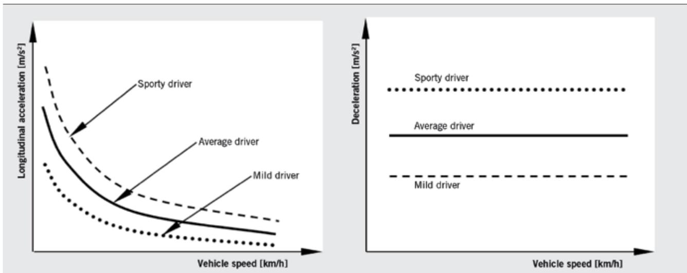
④ Reference samples regarding the correlation of longitudinal acceleration and deceleration to the vehicle speed
