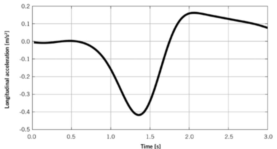
3 Characteristic curve of longitudinal acceleration during a transmission downshift
