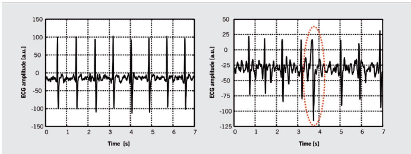
7 Extra systole (right) and sinus rhythm of a healthy driver (left) measured with capacitive electrodes
