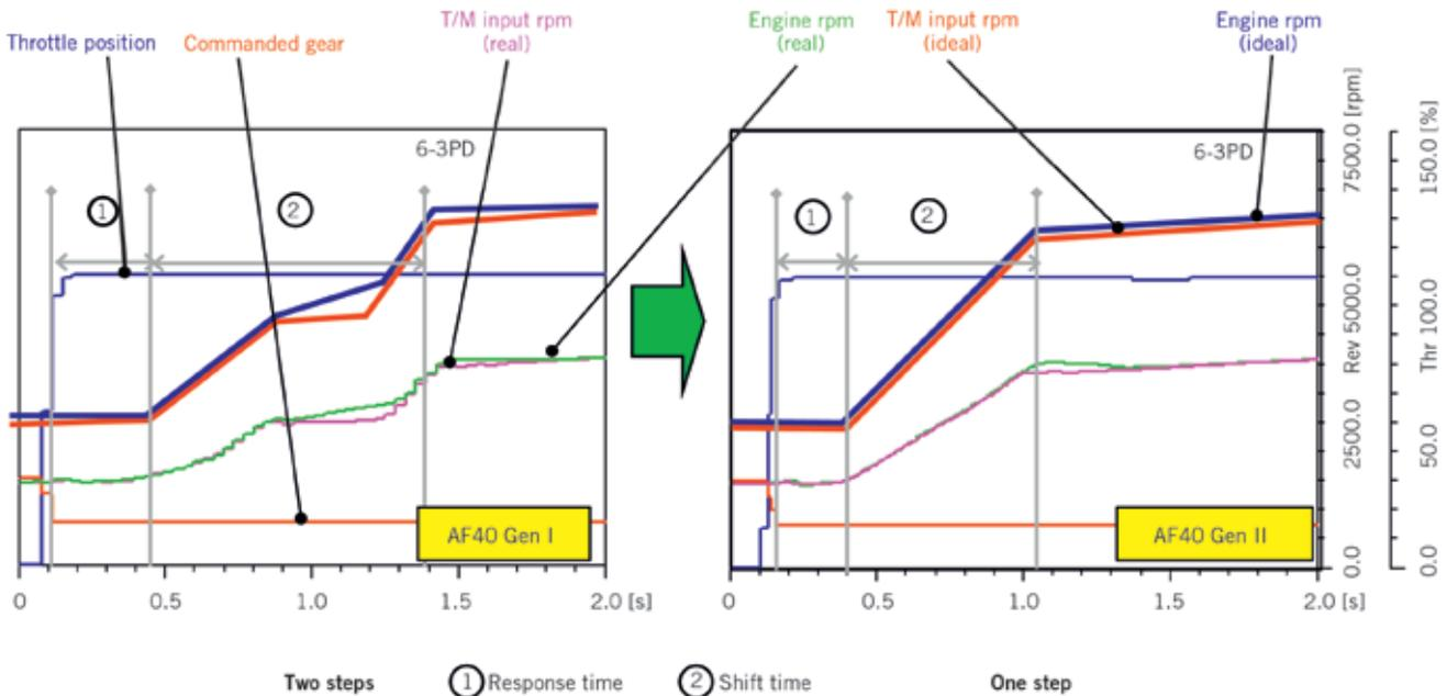
6 Time diagram for shift comfort improvement by eliminating the two-step response behavior with the new transmission
