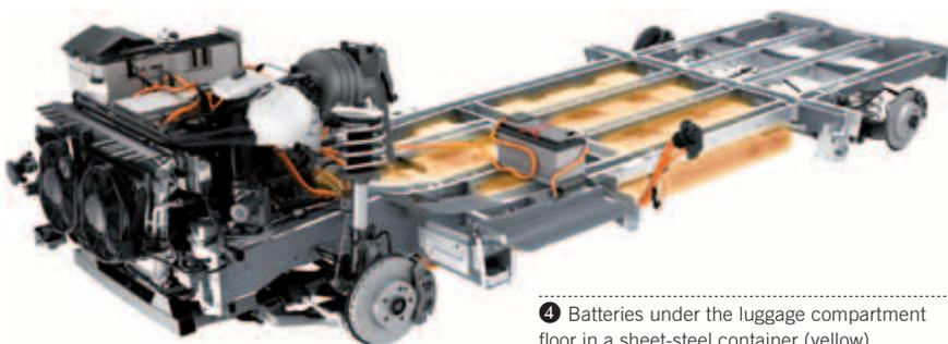
④ Batteries under the luggage compartment floor in a sheet-steel container (yellow)
