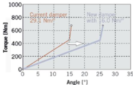
④ New torque converter with longer travel damper compared to the current design
