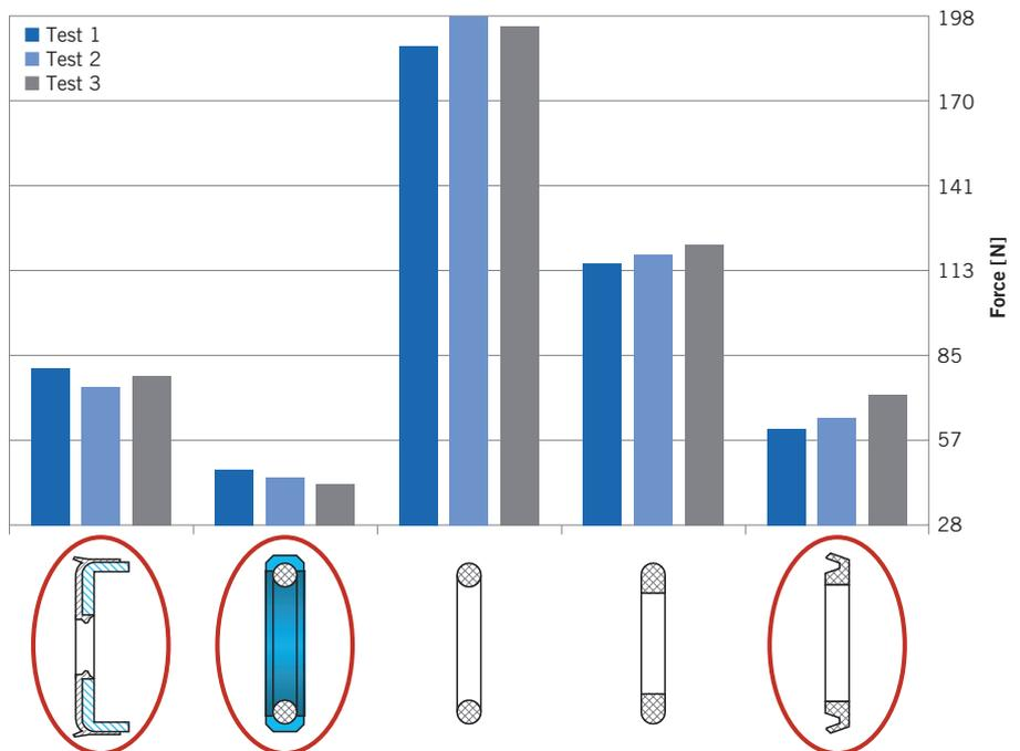
❶ Basic tests with different transmission piston seals reveal big differences in their friction behavior – the solutions, which have so far delivered the best results, are marked in red (from left to right: composite transmission piston seal, a combination of O-ring with PTFE slip ring, O-ring, D-ring, as well as a U-packing; measurements of maximum friction at 500 mm/min, 5 bar sealing pressure and 23 °C)
