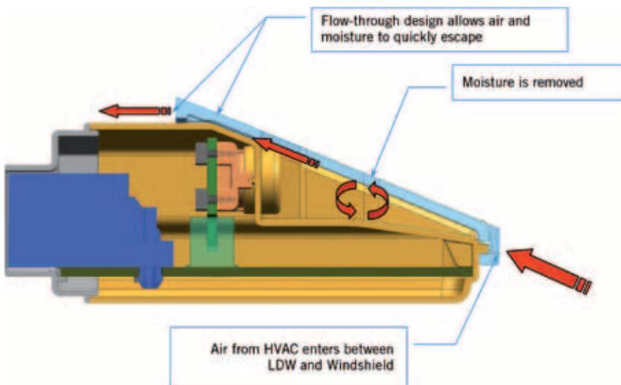
7 Air flow concept in order to remove possible moisture in front of the camera
