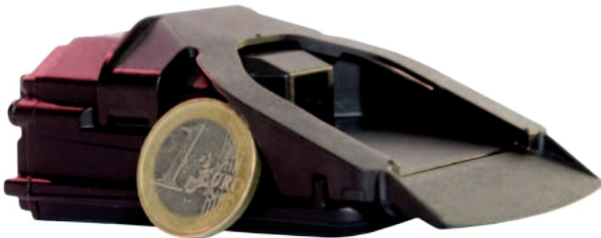
❶ TRW S-Cam: multifunctional sensor supporting an array of driver assistance and safety functions in a single unit
