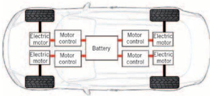
④ Drive-train based on four decentralized electric motors
