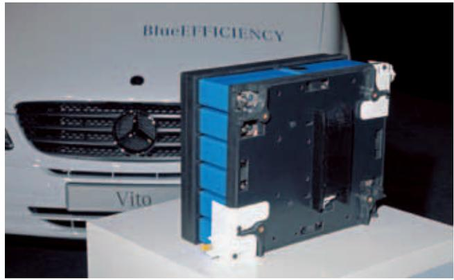
③ Lithium-ion batteries with an energy capacity of 36 kWh
