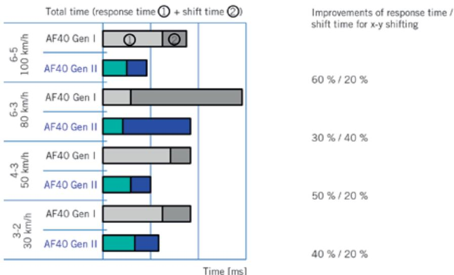
⑤ Response time and shift time comparison for the current and the new transmission for four x-y down shiftings
